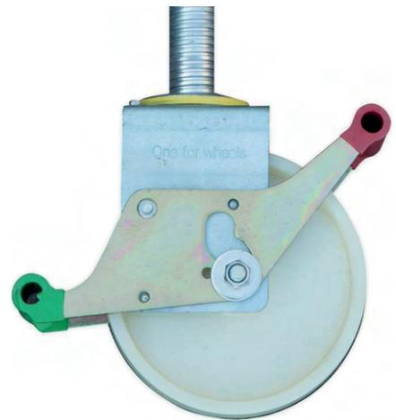
Ø 200 mm swivel castor made of nylon or rubber with spindle. The spindle is adjustable up to a height of 30 cm. Three types of castors are available, 300, 500 and 800 kg load per castor.
